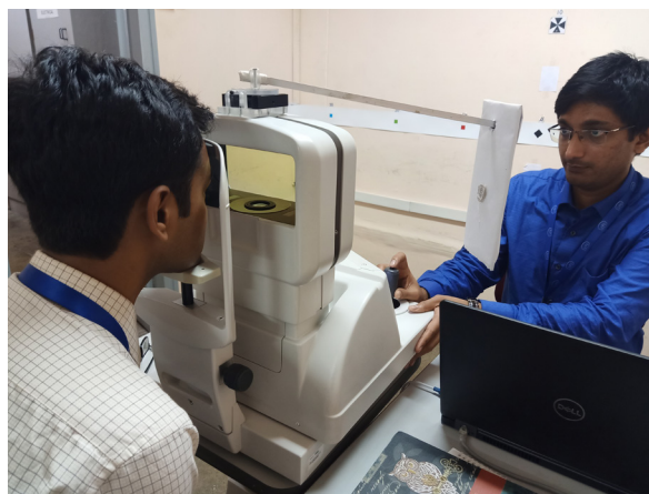
Open-field auto-refractor to determine peripheral refraction. INDIA
